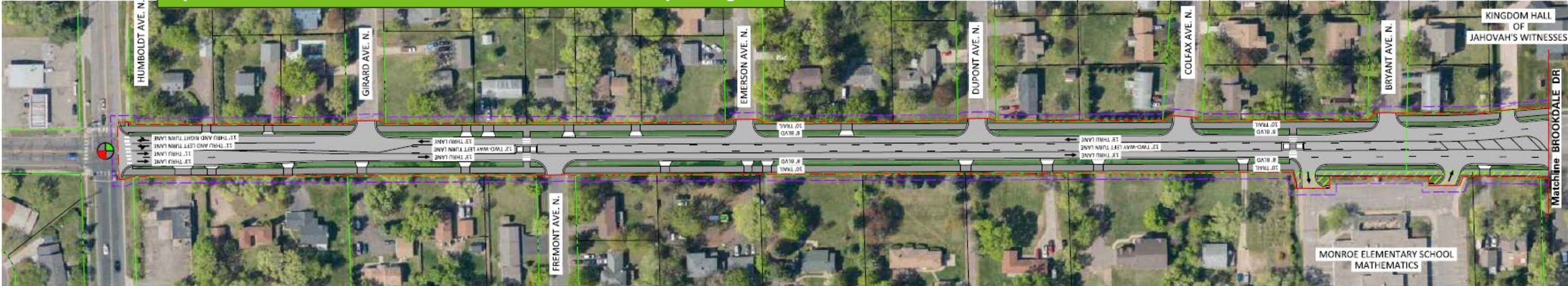
Option A – Two lane with center left turn lane and no parking
