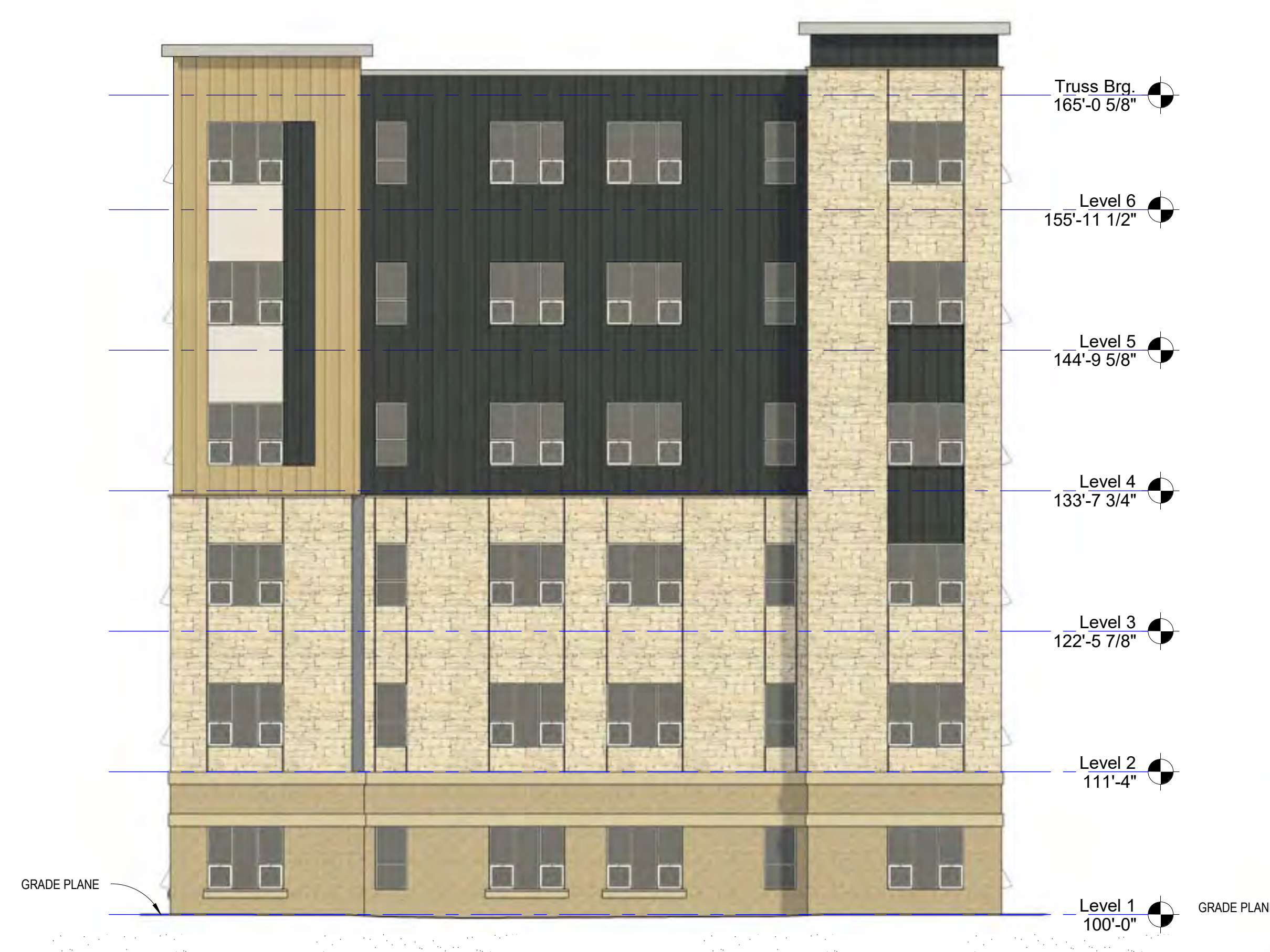
2 Building A Elevation 8 1/8" = 1'-0"
