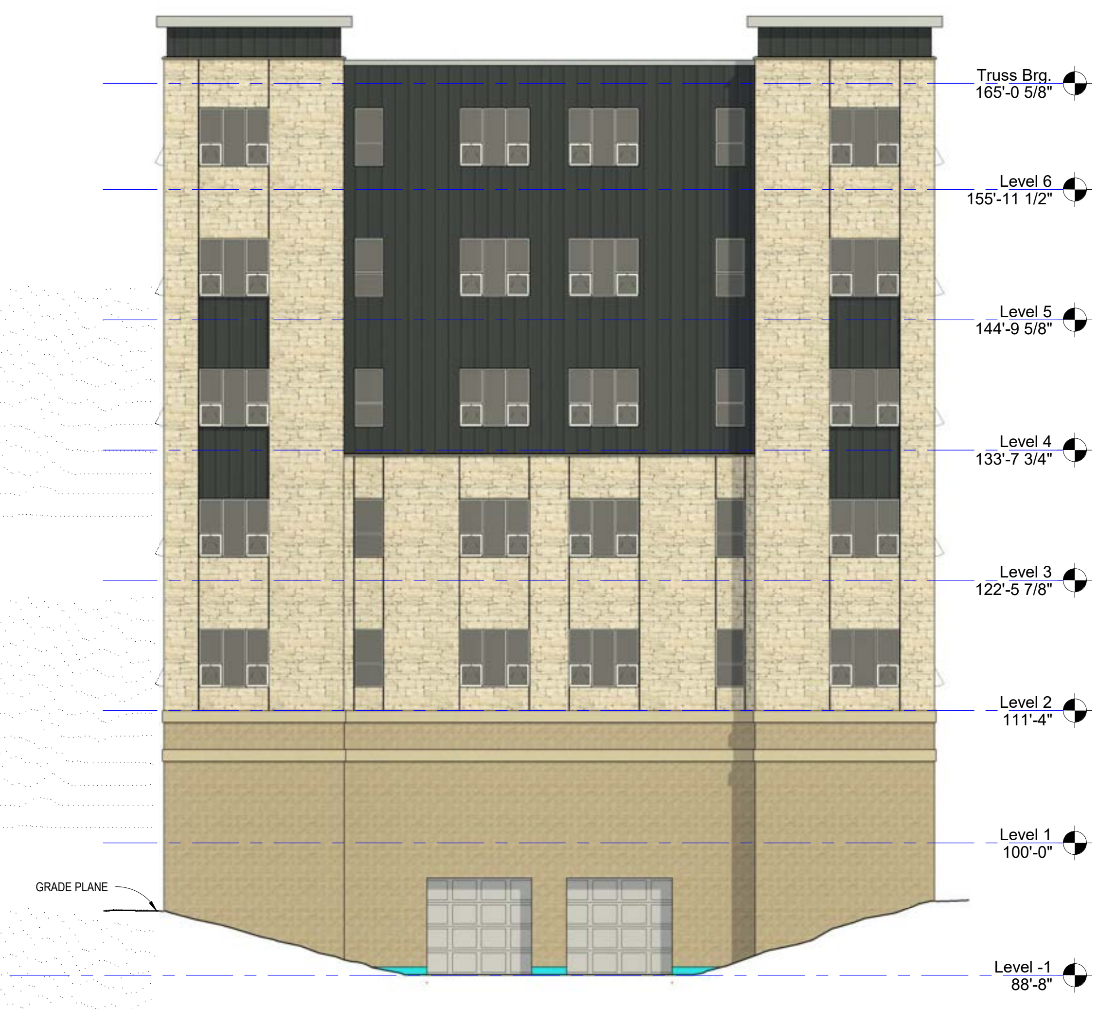
3 Building A Elevation 6 1/8" = 1'-0"
