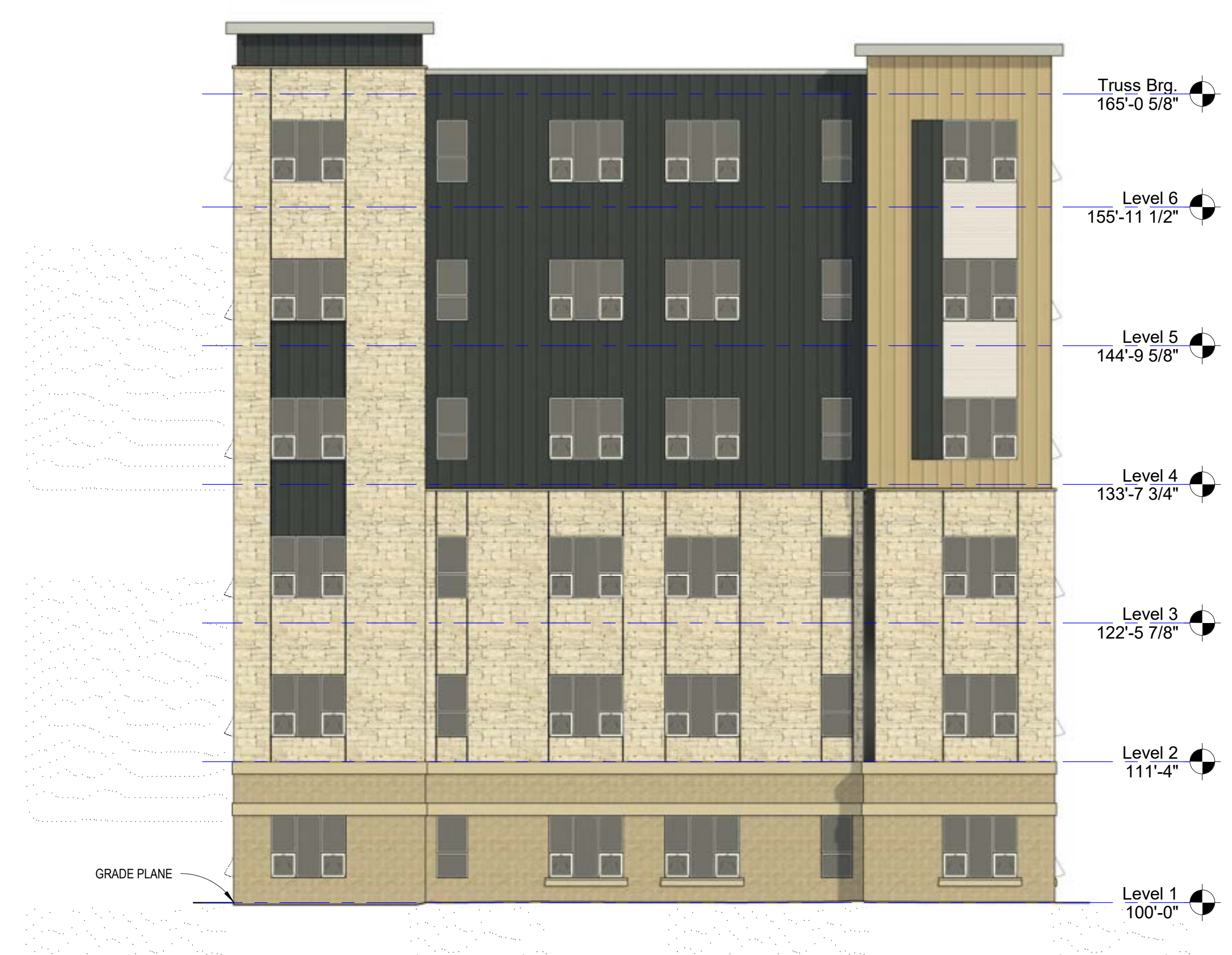
③ Building B Elevation 6 1/8" = 1'-0"
